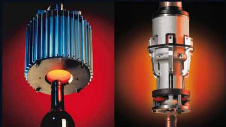
PVC capsules thermoshrinking
